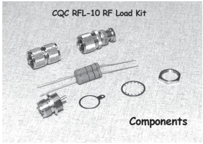
The CQC RFL-10 RF Load project consists of two 5W 100-ohm metal oxide resistors that are connected in parallel to an SO239 coaxial socket. The kit includes adaptors for connection of the Load to either an SO239 or BNC antenna socket. The RFL-10 will handle up to 10W continuous power for at least 60 seconds, with flat SWR across the HF spectrum.
