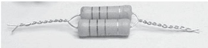
**3. Bend one pair of twisted leads down**, toward the center of the resistor bodies and then down again to make an “S” shape. Bend the other pair of leads straight down.
