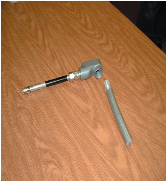
Scratch built hardline connector using common electrical conduit pieces. Display items curtesy of Steve Finch, AI0W
