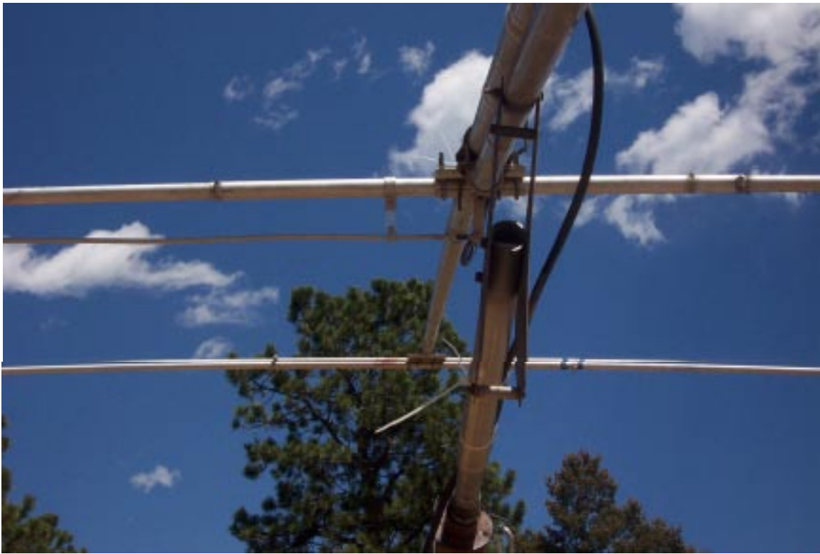
The tilting boom to mast on the 20m yagi built by K9AY
