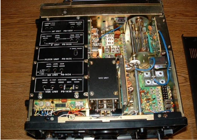
Inside look at a FT-301. All major block components are mounted on plug-in PCB boards. This allows for ease of service and replacement.
