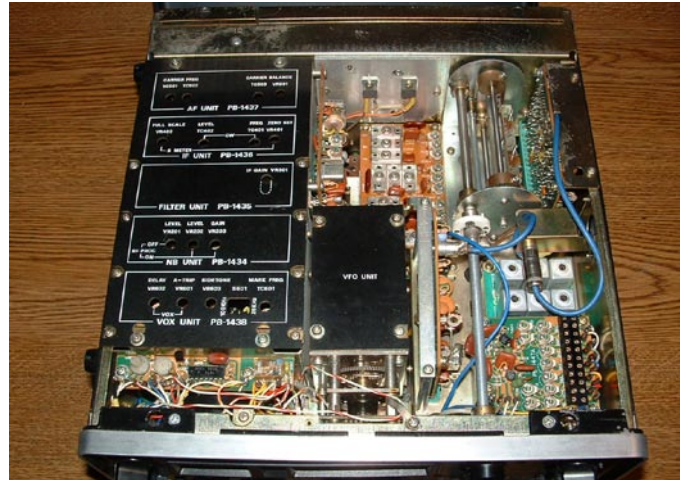
An FT-301SD, similar to the high power unit. Major difference is the lack of the final power amp replaced by the 2 final transistors on the back of the chassis. S units are not equipped with a full compliment of band crystals. 160 ,upper 10M and WWV/JJV 5mhz crystals and not installed. Also speech processor is not enabled.
