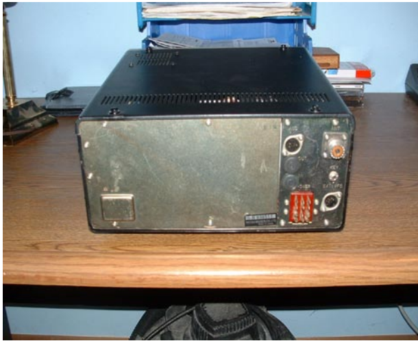
Back view of an FT-301SD. Notice the lack of the power brick and the BNC connections. This unit can not be made into a high power unit. When purchasing one of these don't forget the power connector. It's quite unique.
