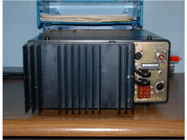
Same view of an FT-301 high power unit. This unit can be run QRP by removing the power brick and jumping the BNC connectors. Antenna connects to the SO-239 connector for use by the transmit/receive relay.
